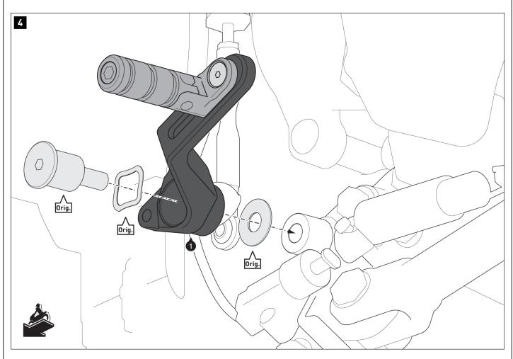
Screw the gear lever [1] with the original parts (Orig.) to the vehicle. **A WARNING:** Use a liquid threadlocker! Tighten the original screw (Orig.) according to the manufacturer's instructions.
