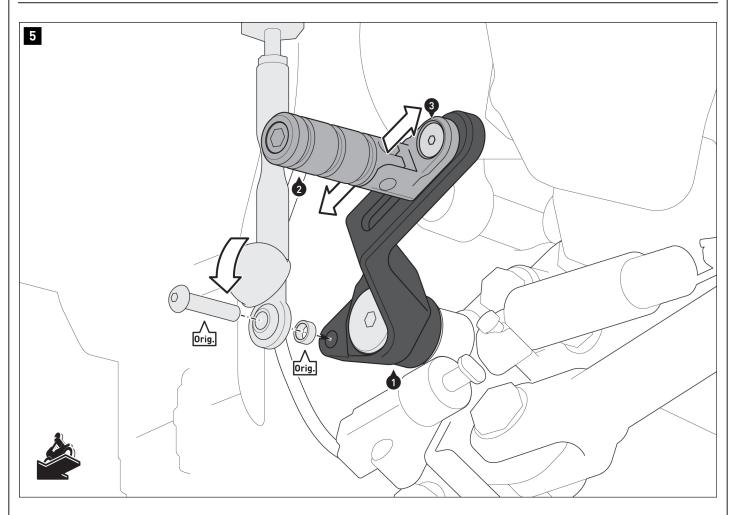
Screw the gear lever (1) to the shift rod.
