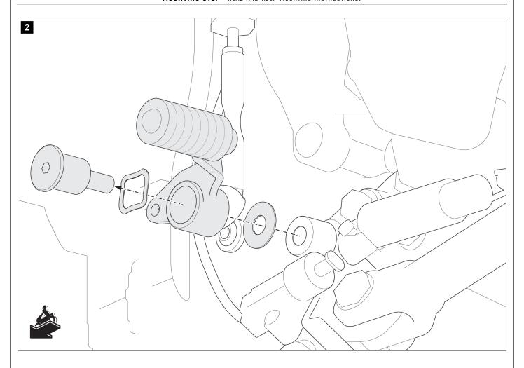
Loosen the parts shown; remove the original gear lever from the vehicle.
