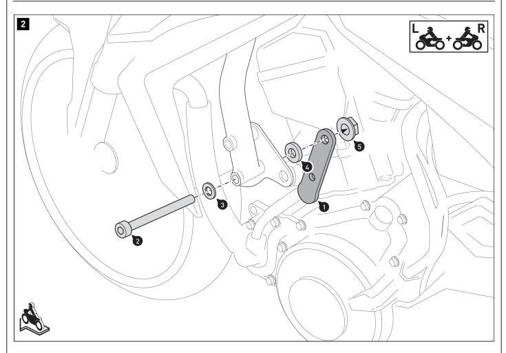
Screw the mounting bracket (1) to the vehicle. Do not tighten the screw yet.
