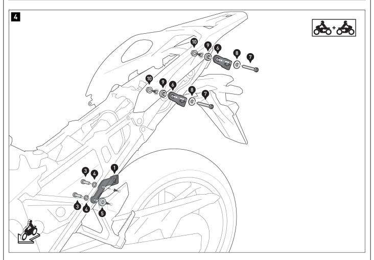
Screw fastening clips (1), (2) and (6) to the vehicle on both sides. The nuts (10) must be positioned on the inside of the passenger grab handles. **A WARNING:** Use liquid thread locker (only the screws (3))! Do not tighten the screws yet.
