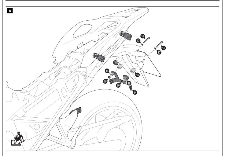
Screw the crossbar (14) to the license plate on the license plate holder. Do not tighten the screws (16) yet.
