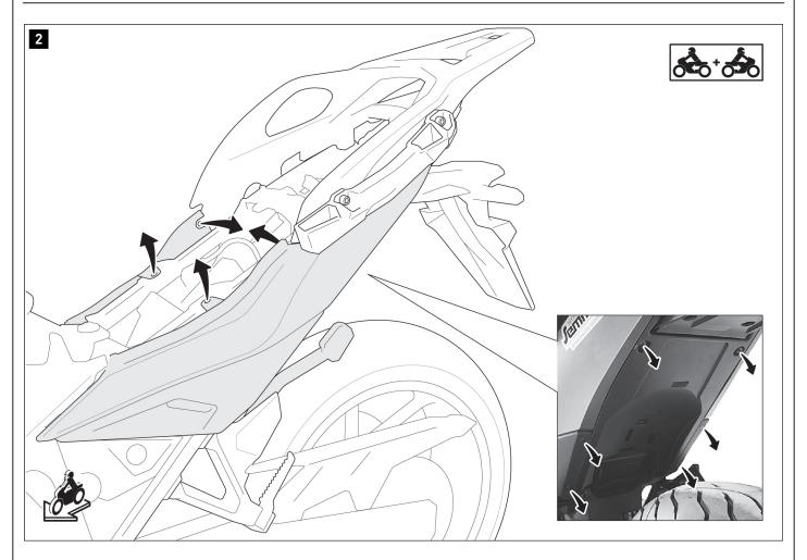
Loosen the indicated screws and plastic anchors of the left and right rear panels.
