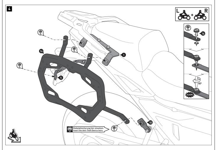
Connect the side carriers (14) and (15) with the quick-release fasteners (16) to the mounting brackets (1), (10) and the crossbar (5). Secure the quick-release fasteners using the lock washers.
