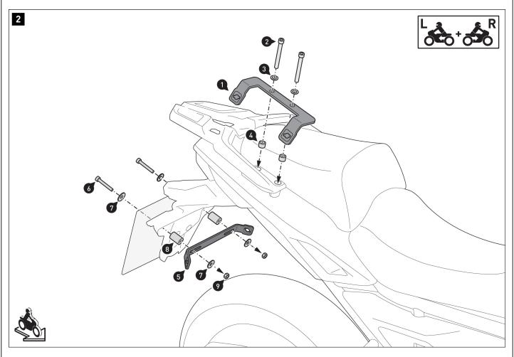
Screw the mounting brackets (1) to both sides of the rear of the vehicle. **A WARNING:** Use liquid threadlocker!
