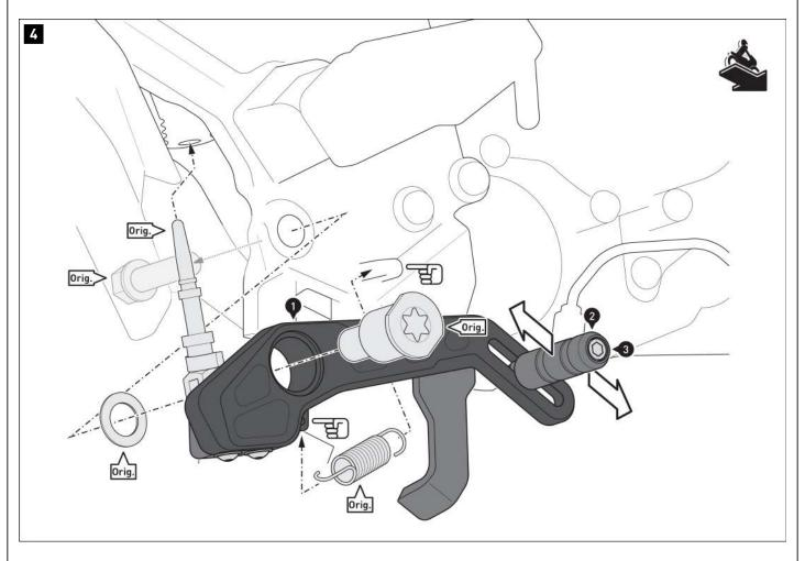
Insert the original pressure rod (Orig.) into the master brake cylinder.
