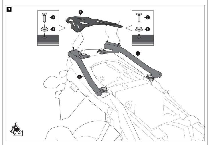
Screw the rack (6) to mounting struts (1) and (2). **A WARNING: Use a liquid threadlocker!**
