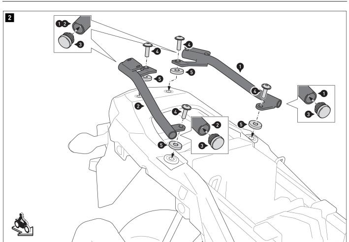
**NOTE:** If you are installing the SW-MOTECH side carrier at the same time, spacers (5) are not required. Mount the side carrier and crossbar in their place.
