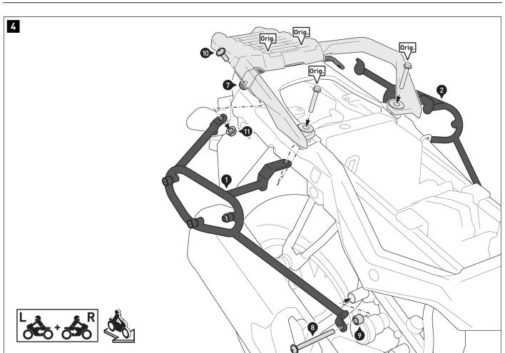
Screw side carriers (1) and (2) to the vehicle and to the crossbar (7). Be sure to screw side carriers (1) and (2) to the rear mounting points located **under** the crossbar (7).
