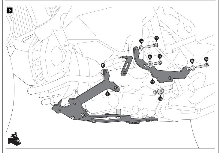
Screw the left mounting bracket [12] onto the vehicle. **A WARNING: Use a liquid threadlocker!**Do not tighten the screws yet.
