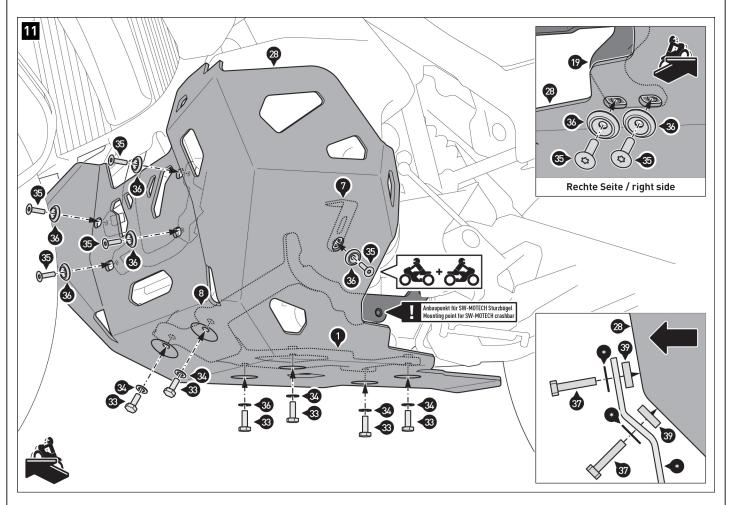
Screw the engine guard [28] onto the mounting supports, mounting brackets, and the front mounting points.
