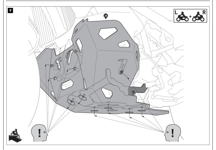
With the help of a second person, press the engine guard (28) onto all previously mounted mounting supports, mounting brackets, and the front original mounting points.
