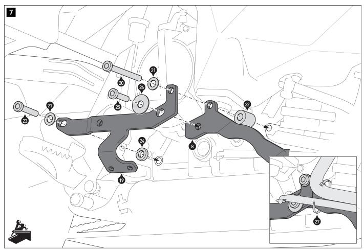
Screw the right mounting bracket (19) onto the vehicle. **A WARNING:** Use a liquid threadlocker!
