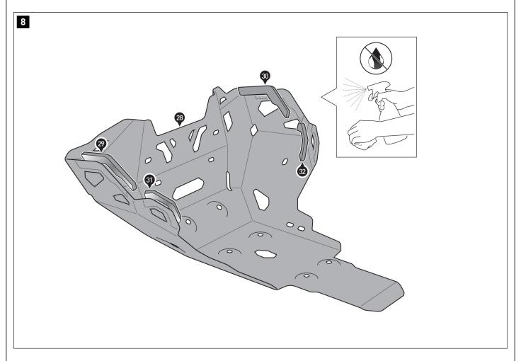
Thoroughly clean the surface of the engine guard (28) to remove any grease and dirt residue.
