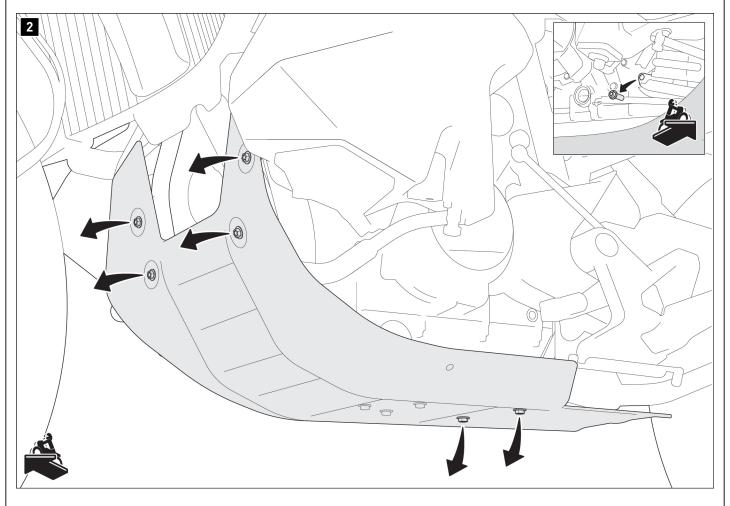
Remove the original screw (see detailed image) on the right side of the vehicle.
