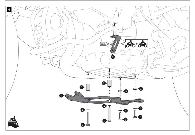
Screw the lower mounting plate (1) and the mounting support (7) to the vehicle.
