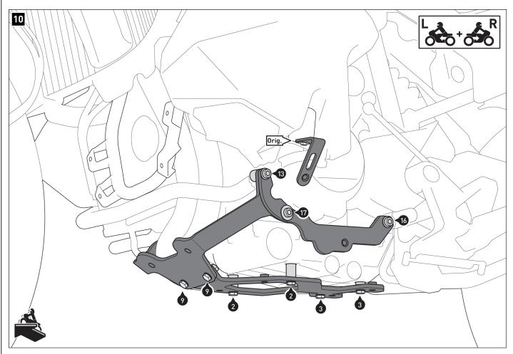
Tighten the screws in the following order: (13), (16), (20), (23), (2), (3), (17), (25), (9), (0rig.).
