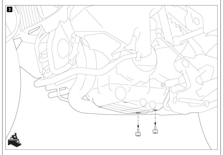
Remove the original rubber dampers shown.
