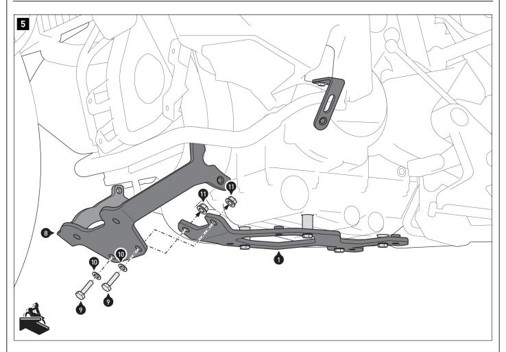
Screw the front mounting bracket (8) to the mounting bracket (1). Do not tighten the screws yet.
