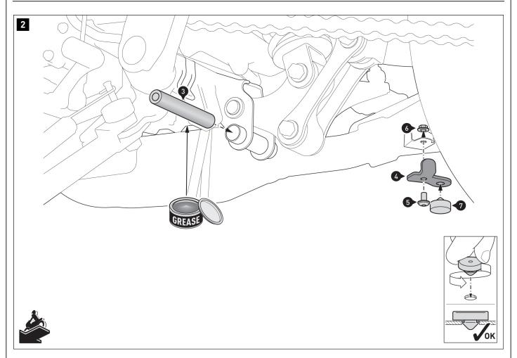
Coat the outside of the bearing bush (3) with grease.
