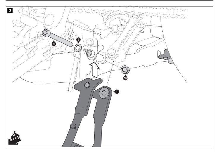
Screw the centerstand (1) to the vehicle. Tighten the screw (8) as specified in the mounting instructions.
