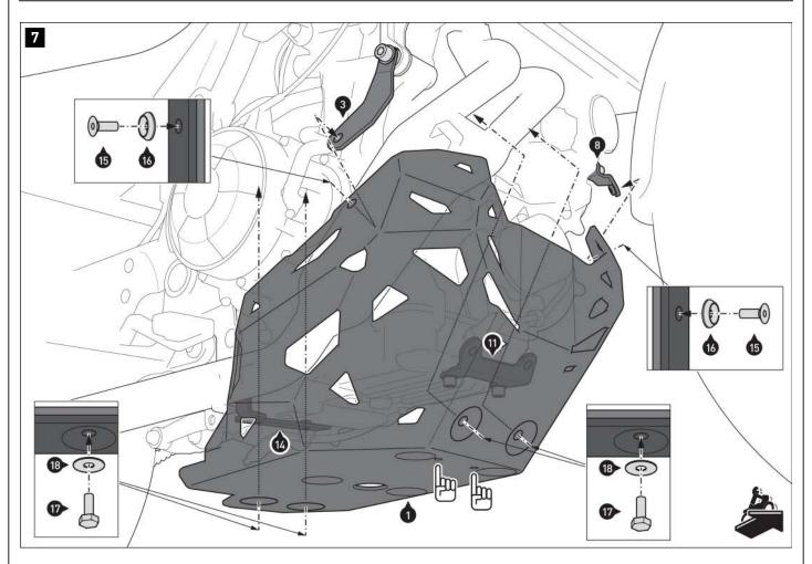
Screw the engine guard (1) to the mounting brackets (3), (8), and (11) and the crossbar (14).
