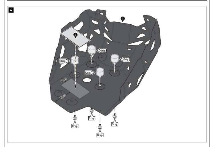
Thoroughly clean the marked surface of the engine guard (1) to remove grease and dirt residues.
