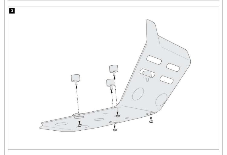
Remove the four rubber dampers from the original engine guard.
