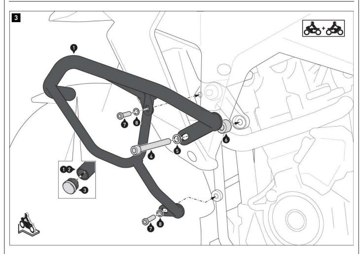
Insert the plastic plugs (3) into the openings on the crash bars (1) and (2) as shown in the detail drawing.
