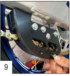
Place the 2 TFHC 6x60mm in the bottom holes using M6 washers and EM6F bolts.
