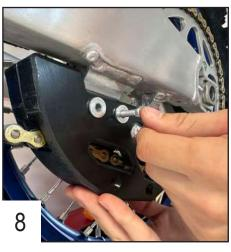
Place the TH 6x60mm in the 2 top holes using the EM6F bolts.
