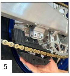
Place the small part behind the chain and slide to align it to the swingarm holes.
