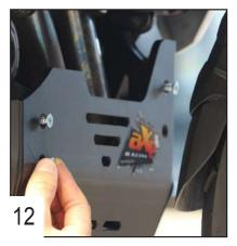
Place the 2 other front TFHC 6x35mm screws. Do not tighten.
