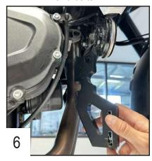
Put the front fixations in place, the clamped bolts must face the outside.
