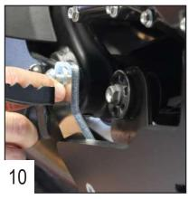
Put the TBHC 8x25mm + M8 washer and EM8F bolt in the rear right fixation. Do not tighten.
