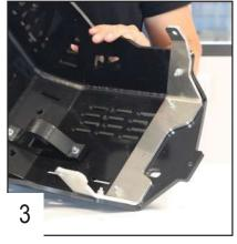
Place the rear alu fixation using 4 TFHC 6x25mm screws + washers and bolts.
