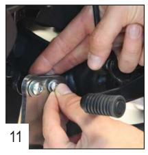
Put a TBHC 8x25mm + M8 washer and EM8F bolt in the biggest hole of the rear left side. And a TBHC 6x25mm + M6 washer and EM6F bolt in the small hole. Do not tighten.
