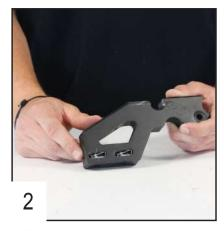
Place 2 clamped bolts in each front fixation.
