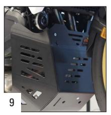
Place 2 front TFHC 6x35mm screws without tightening to maintain the skid plate in the correct position.
