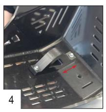
Place the center plastic block using 2 TFHC 6x30mm screws + washers and bolts then tighten.
