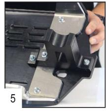
Place the rear plastic block using one TFHC 6x50mm screw in the biggest hole and 2 TFHC 6x30mm screws + washers and bolts.
