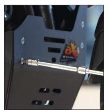
Pass the hoses through the hole at the rear of the skid plate.
