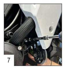
Use one TBHC 8x40mm screw + M8 washer and EM8F bolt on each side.
