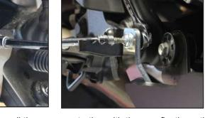
Tighten all the screws; starting with the rear fixations, then the front screws.
