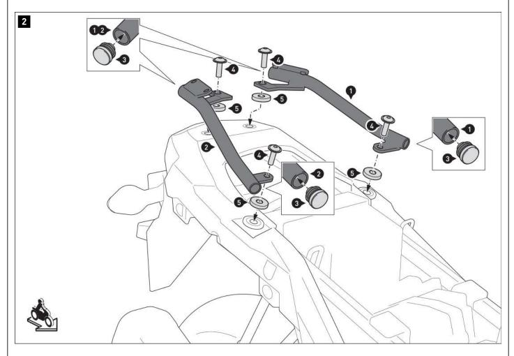
$\triangle$  **NOTE:** If you are installing the SW-MOTECH side carrier at the same time, spacers (5) are not required. Mount the side carrier and crossbar in their place.
