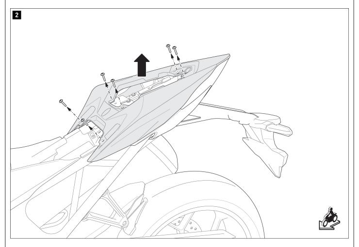
Loosen the original screws, and remove the fairing from the bike.
