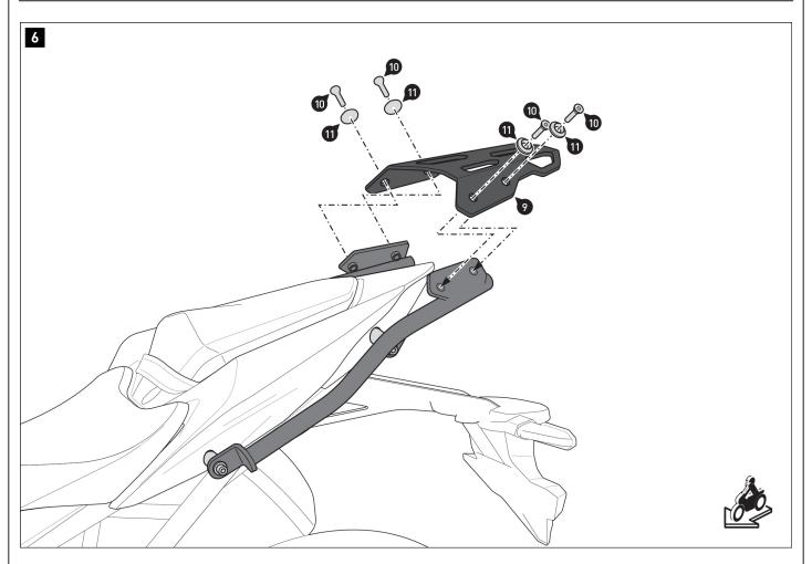
Screw the rack (9) onto the mounting struts (1) and (2).
