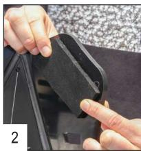
Cut the foam in two pieces and stick one to the inside top of each side of the skid plate.
