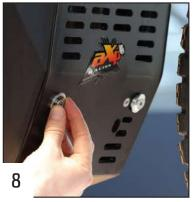
Use 2 alloy spacers + 2 TFHC 8x30mm screws to fix the front of the plate. Do not tighten yet.
