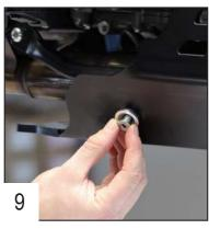
Place one alloy spacer + 1 TFHC 8x30mm screw on each side of the plate.
