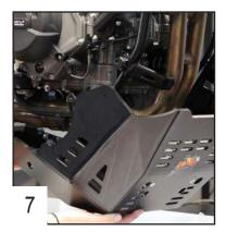
Place the plate under the bike and clip the rear bracket on the frame tube.
