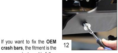
Remove the rear screws and the spacers.
