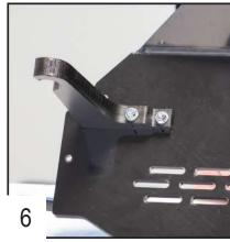
Place the rear bracket, make sure to use a TFHC 6x30mm screw in the longest hole and a TFHC 6x25mm screw in the smaller one + M6 washers and bolts.
