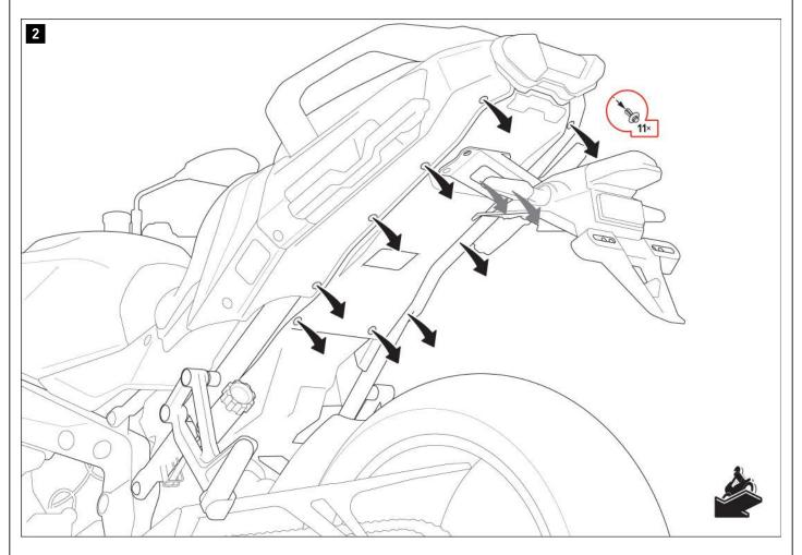
Remove the marked plastic dowels from the rear panel. Pull the back of the rear panel down slightly.
