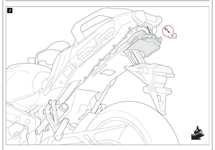
Loosen the indicated screw and remove the fairing from the vehicle.
