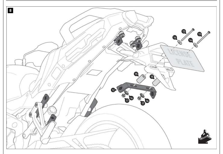
Screw the crossbar (12) onto the license plate holder. Do not tighten the screws (13) yet.
