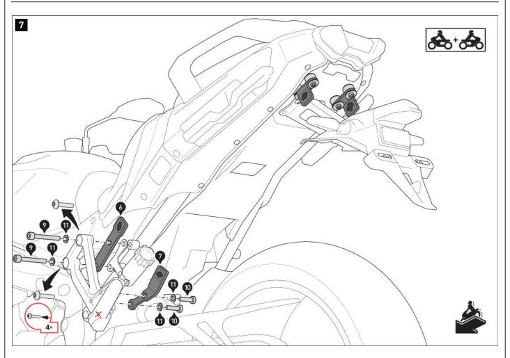
Remove the four passenger footrest bolts from the vehicle.
