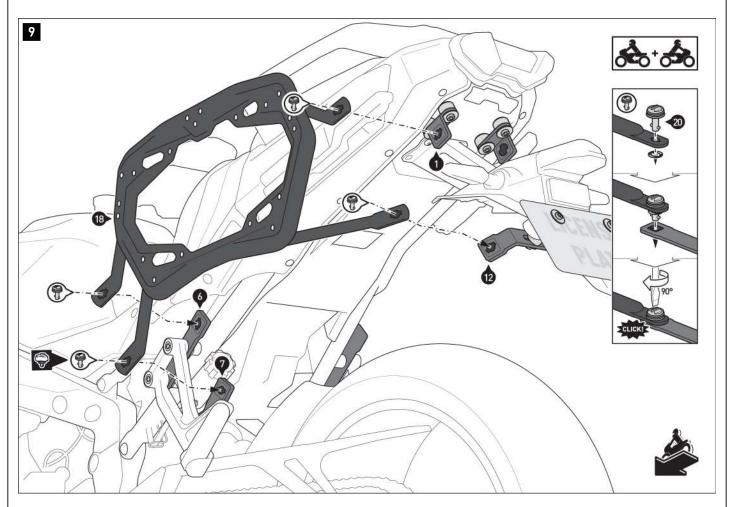
$\triangle$  **NOTE:** SW-MOTECH anti-theft protection is sold separately; mount the anti-theft protection onto **both sides** of the vehicle as indicated.
