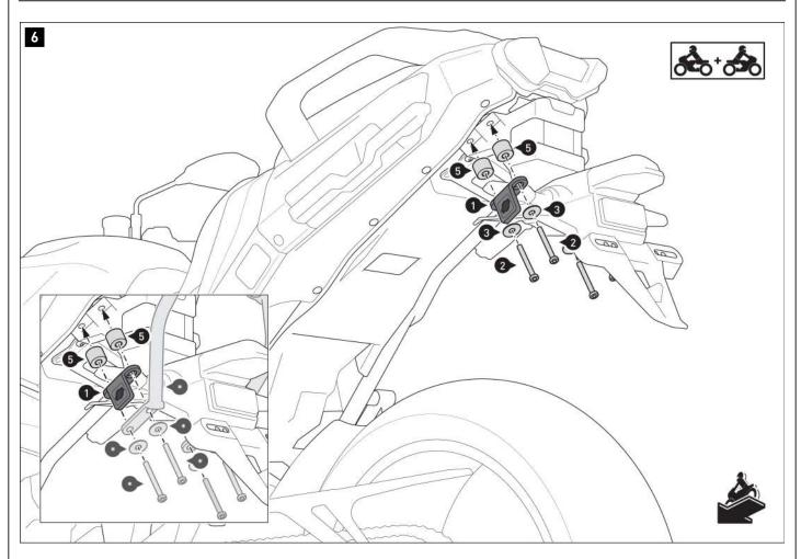
$\triangle$  **NOTE:** The detailed drawing illustrates how to mount the side carrier with the SW-MOTECH rack. Use the mounting parts included with the rack (\*) together with the indicated parts for the side carrier.
