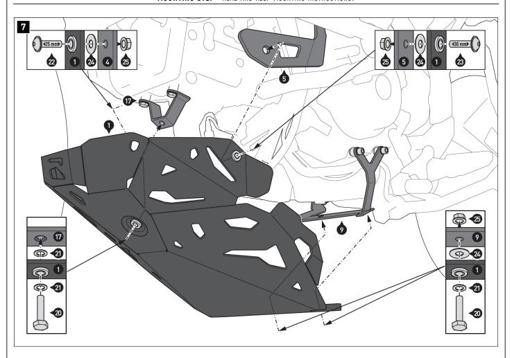
When all components are loosely attached, tighten all screws as specified in the mounting instructions. Concealed screws can be tightened through the recesses in the engine guard.
