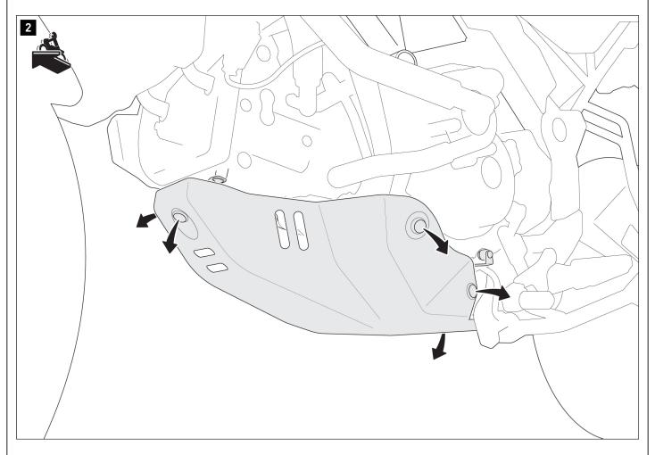
Loosen the indicated screws on the original engine guard. Remove the engine guard from the vehicle.
