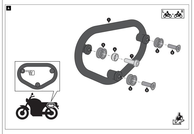
Screw parts (5) to (8) to the side support (1). **A** WARNING: Use liquid threadlocker!
