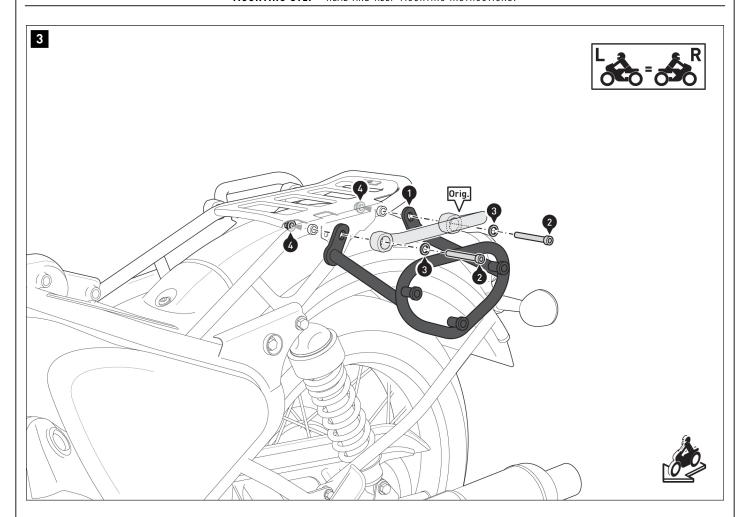
Screw the side carrier (1) to the original passenger grab handle (Orig.) on the vehicle.
