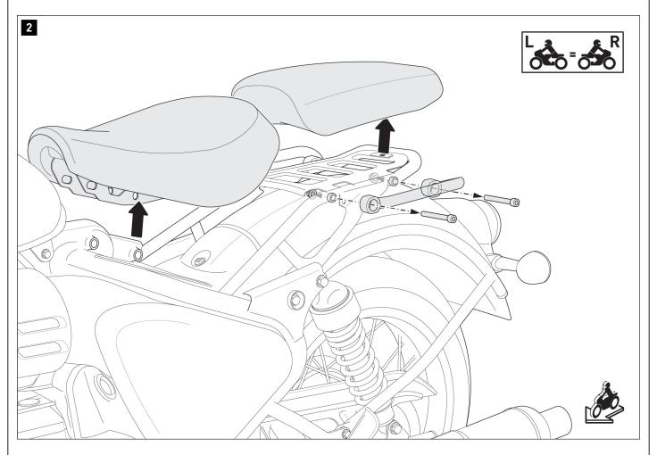
Remove the seats and original parts shown from the vehicle.
