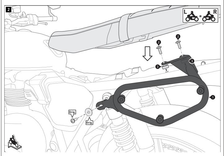
Screw the side carrier (1) to the vehicle using the original parts (Orig.).
