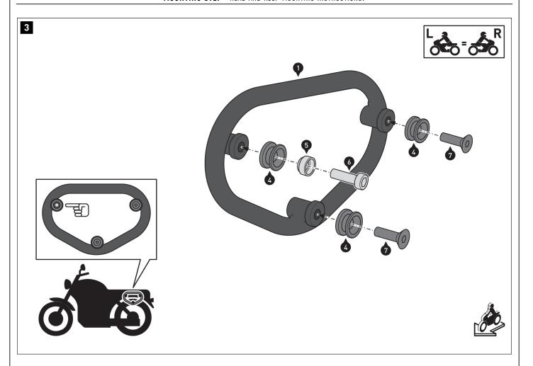
Screw parts (4) to (7) to the side support (1). **A** WARNING: Use liquid threadlocker!
