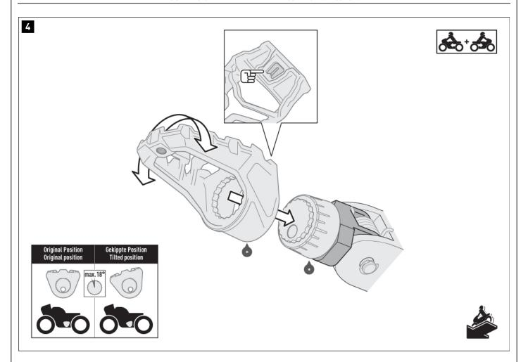
Place the footrests (\*) onto the positioning cones (\*). By interlocking the positioning cones (\*), the angle of inclination of the footrests (\*) can be individually adjusted (no more than 18°; see detailed drawing on the left).
