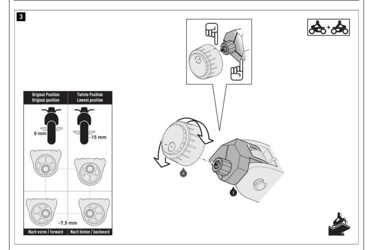
Place the positioning cones (\*) onto the star-shaped mounting cones on the joint adapters (1/2). Thanks to the different mounting positions, the height of the footrests (\*) can be individually adjusted (see detailed drawing on the left).
