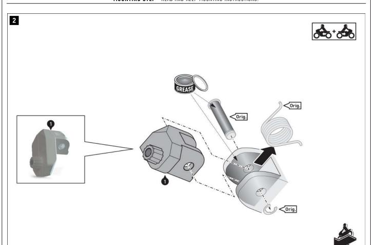
Clean the footrest mounts thoroughly. Apply some grease to the inside of the footrest mounts as well as to the original bolts (Orig.) .
