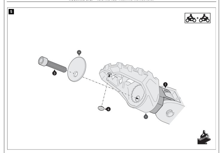
First, loosely screw the footrests (\*) to the joint adapters (1/2). Check again for side-synchronous alignment and ergonomics.
