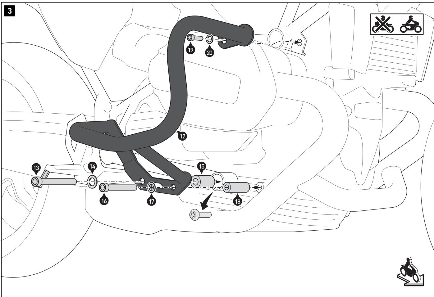
Remove the original engine mounting bolt on the **right** side of the bike.
