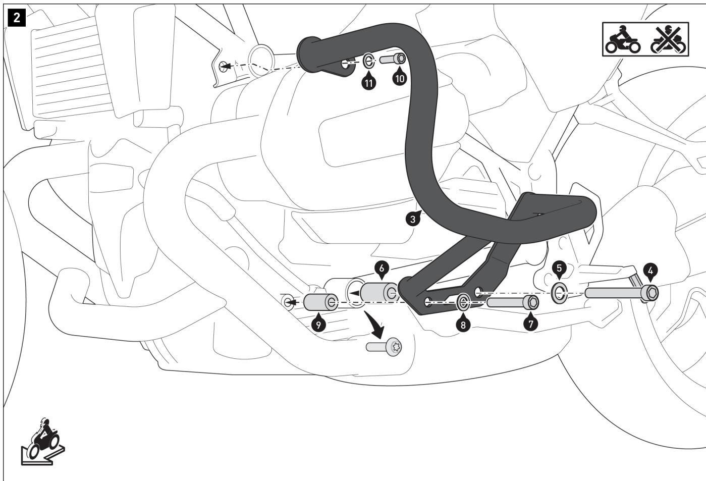
**⚠ WARNING: Do not start installing the right crash bar until you have completed installing the left crash bar!**
