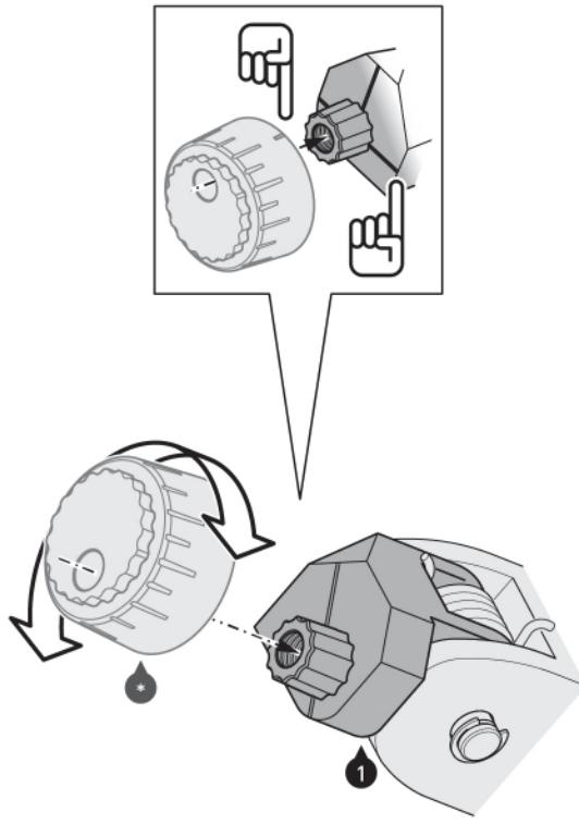
Place the positioning cones (1) onto the star-shaped receiving cones of the joint adapters (1/2). Because of the different mounting positions, the height of the footrests (1) can be individually adjusted (see left detailed drawing).
