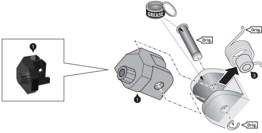
Clean the footrest mounts thoroughly. Apply some grease to the inside of the footrest mounts and the original bolts (Orig.).
