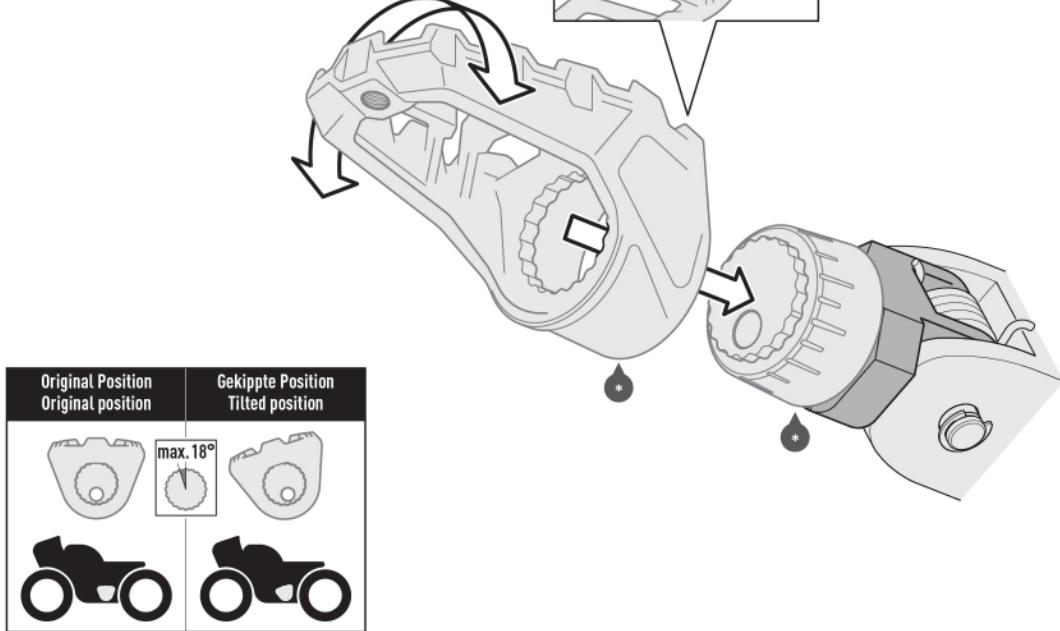
Place the footrests (·) onto the positioning cones (·). By interlocking the positioning cones (·), the angle of inclination of the footrests (·) can be individually adjusted (not more than 18°; see left detailed drawing).
