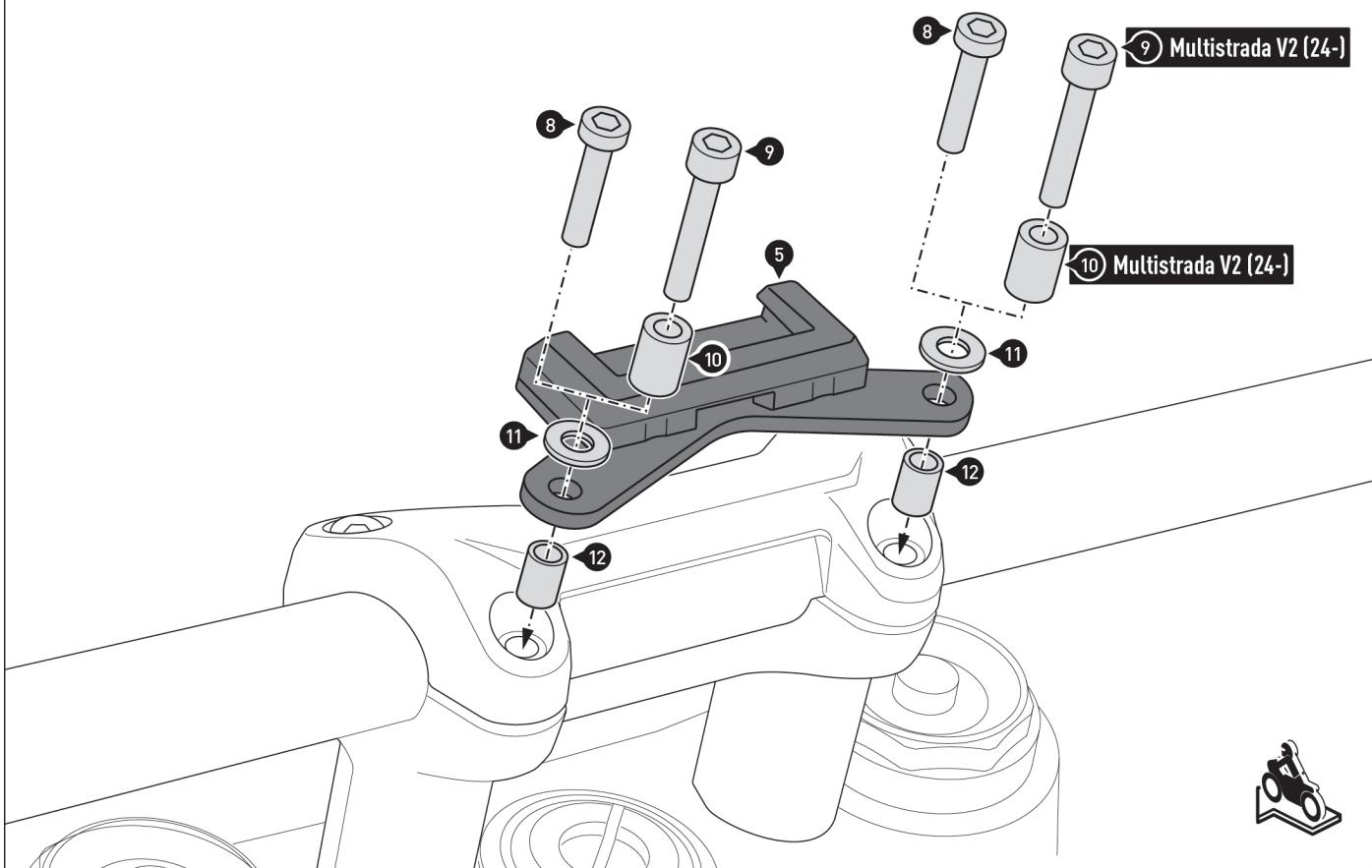
**⚠ NOTE:** For the vehicle model **Multistrada VS (24-)** use **screws (9)** and **spacers (10)**, instead of **screws (8)**.
