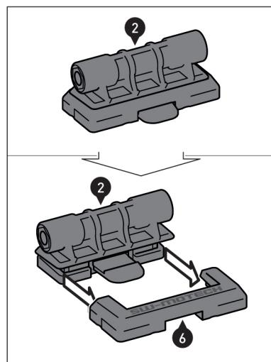
Remove the holding frame (6) from the slide-in frame (2).
