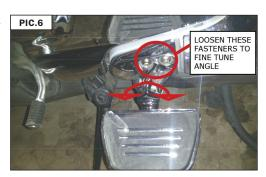
NOTE: If the Mini Boards do not seem parallel after tightening in the desired orientation, they can be fine tuned by loosening the two footpeg mount fasteners and rotating the peg mount forward or backward to achieve the desired position.
