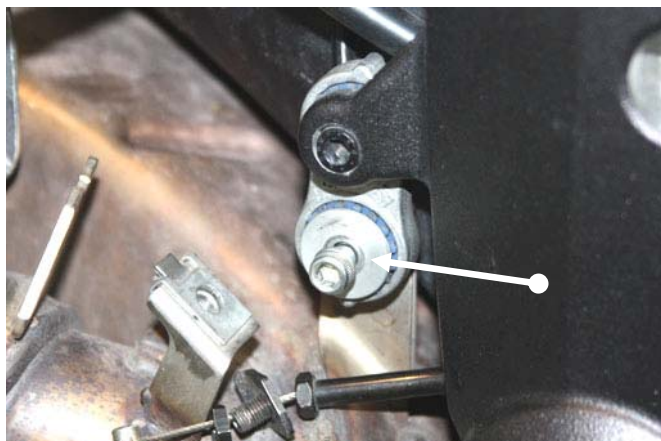
Svitare la vite indicata Unscrew the screw shown in picture
