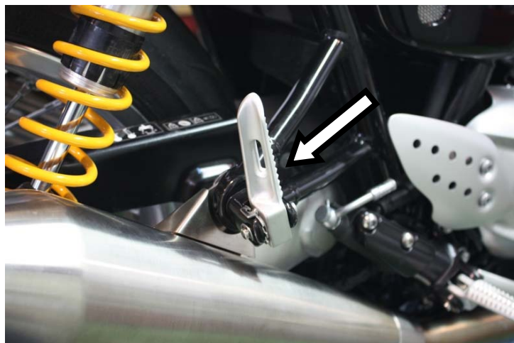
Smontare i pedalini dalle pedane passeggero DX ed SX Remove passengers' footrests, on both sides
