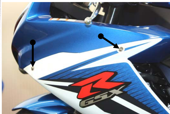
Svitare le viti indicate Unscrew the screws shown above
