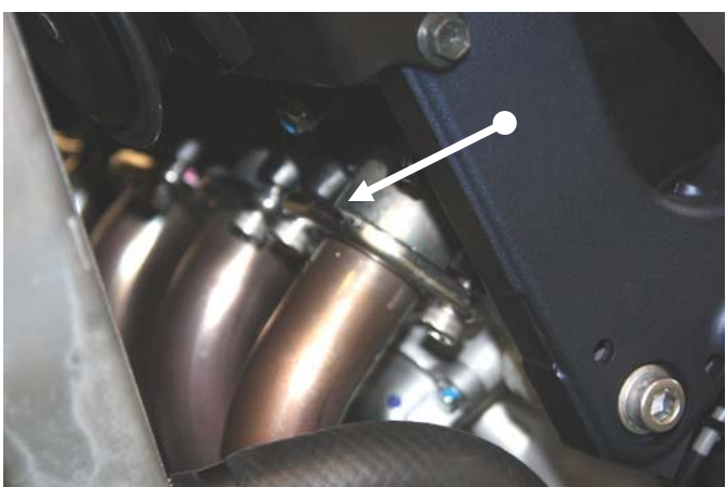
Svitare le viti delle flangie Unscrew the bolts securing the flanges to the cylinders
